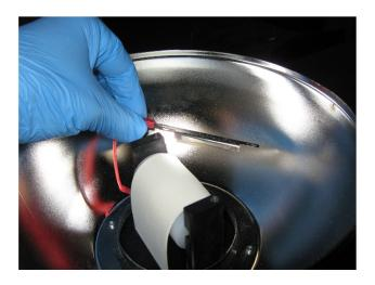
Slide the top roller and the band sideways of the bearings.
