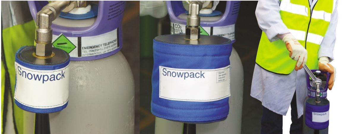
The Snowpack makes individual pellets of dry ice from a carbon dioxide syphon cylinder, which has an internal dip tube.
