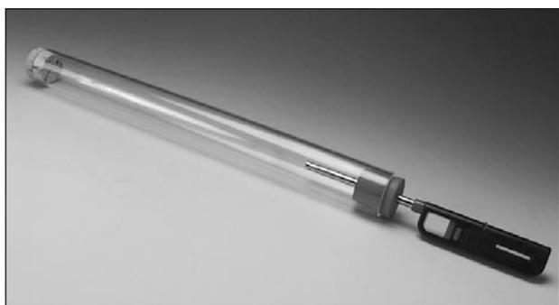
The igniter shall be mounted in the rubber stopper with the large diameter end towards the igniter handle. To reduce friction, a small amount of liquid soap can be applied.
