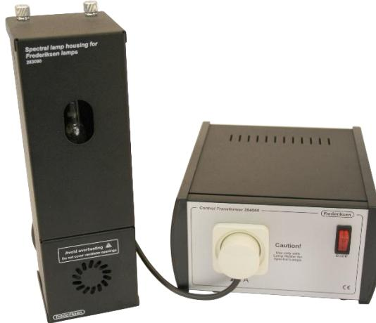
The connector of the spectral lamp housing is connected to the Control transformer in the 3-pin connector on the front. The switch on the Control transformer is switch on and the spectral tube lamp lights up.
