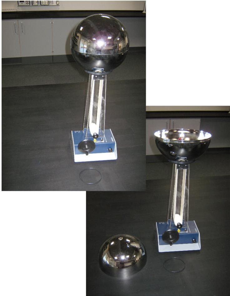
3. Loosen the screw that fixes the lower roller to the steel axle.
