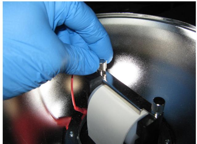
7. Move the comb out of the way. No need to remove the cable.
